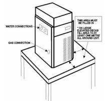
must be installed to fill in the perforations) to prevent excessive drafts entering the water heater from underneath.
